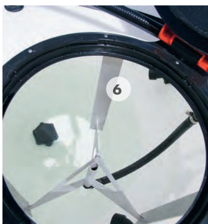
Stainless steel knife to puncture containers combined with rinsing function.
